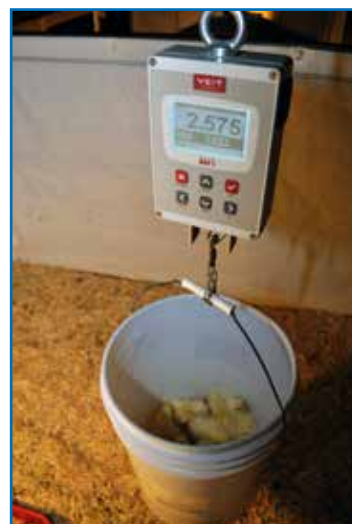
Figure 51: Manual bulk weighing of chicks with an electronic scale.
